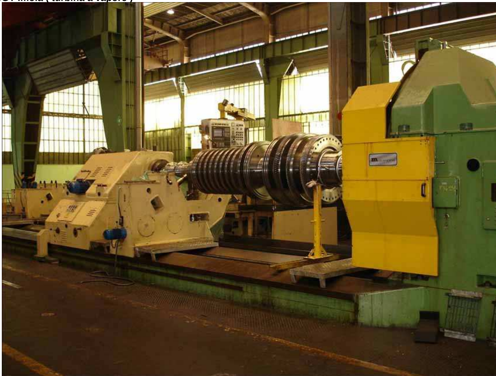
CCGT Imola ( turbina a vapore )
